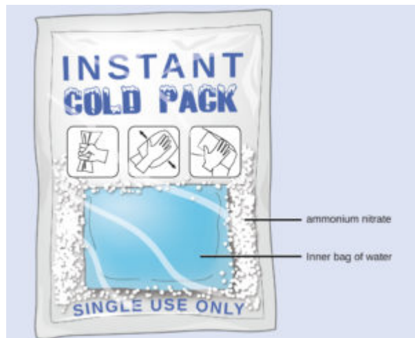
Figure 6 An instant cold pack consists of a bag containing solid ammonium nitrate and a second bag of water. When the bag of water is broken, the pack becomes cold because the dissolution of ammonium nitrate is an endothermic process that removes thermal energy from the water. The cold pack then removes thermal energy from your body.
